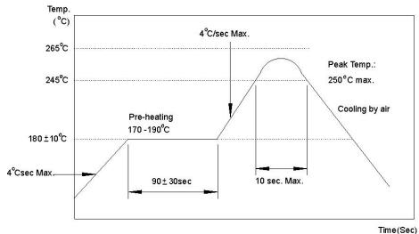
Note: (1) In automated mounting of the SMD sound transducers on PCB, any bending, expanding and pulling forces or shocks against the SMD sound transducers shall be kept minimum to prevent them from electrical failures and mechanical damages of the devices.(2) In the reflow soldering, too high soldering temperatures and too large temperature Gradient such as rapid heating or cooling may cause electrical failures and mechanical damages of the devices.
