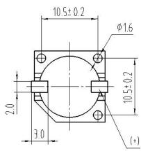
\*Unit: mm; Tolerance:  $\pm 0.5$ mm Except Specified
